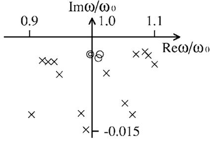
FIG. 3. Resonances of a microstadium cavity. The double and single circles correspond to the resonances of the maximum and second maximum gain.
