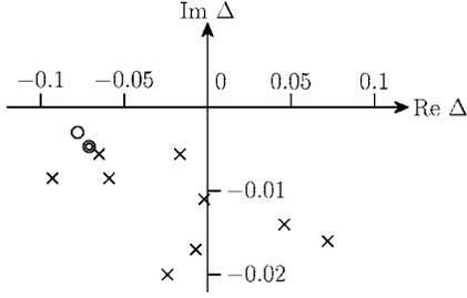
FIG. 6. Resonances of a microstadium cavity. The double and single circles correspond to the resonances of the maximum and second maximum gain.
