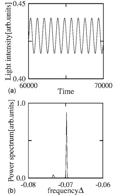
FIG. 11. (a) The light intensity inside the cavity vs time in the case of  $W_\infty = 2.0 \times 10^{-4}$ . The time evolution of the light intensity is quasiperiodic. (b) The optical spectrum has two peaks. The higher peak frequency ( $\nu_1$ ) corresponds to mode A, and the other peak frequency ( $\nu_2$ ) corresponds to mode B.
