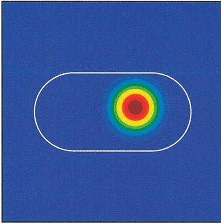
FIG. 8. (Color) The initial state of the light field. The final stationary state does not depend on the initial state. The white curve denotes the stadium cavity.
