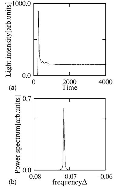
FIG. 13. (a) The light intensity inside the cavity vs time in the case of  $W_\infty = 100 \times 10^{-4}$ . The time evolution of the light intensity grows exponentially at first and exhibits a relaxation oscillation, at last becoming stationary. (b) The optical spectrum has only one peak due to the mode-locking phenomenon.
