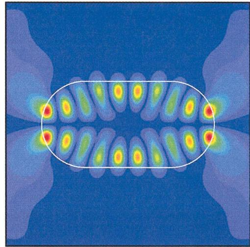
FIG. 10. (Color) The final lasing state of the light field. The wave function corresponds to that of mode A as shown in Fig. 7(a).
