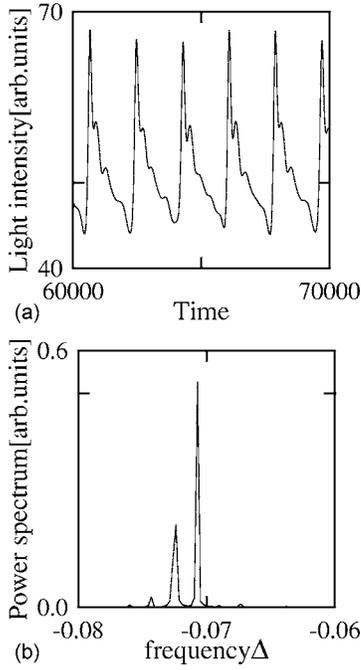
FIG. 12. (a) The light intensity inside the cavity vs time in the case of  $W_\infty = 35 \times 10^{-4}$ . The time evolution of the light intensity is the limit cycle. (b) The optical spectrum has two large peaks corresponding to modes *A* and *B*, respectively, and small peaks of the higher harmonics of the two large peaks frequencies.
