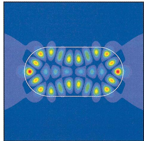
FIG. 5. (Color) The wave function of the resonance of the double circle in Fig. 1. It excellently corresponds to the final stationary lasing state shown in Fig. 3.
