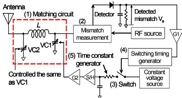
Fig. 1: Configuration of the proposed adaptive matching system
