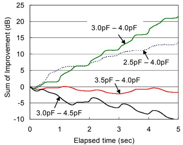
Fig. 4: Effect of the range of capacitance for the varactors on the mismatch improvement
