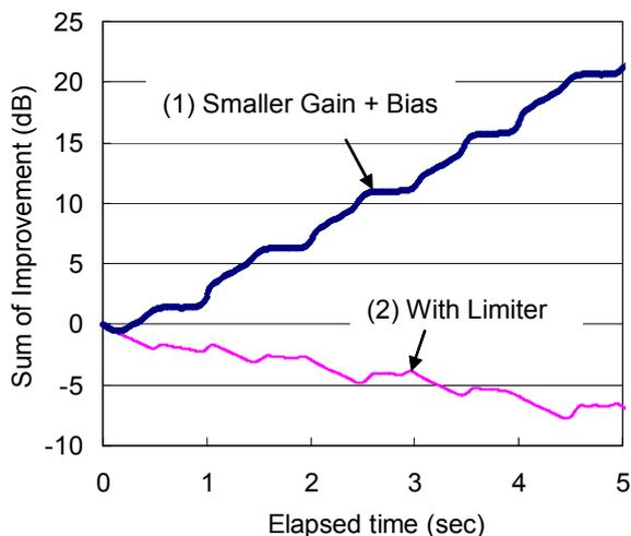
Fig. 5: Time integration of improvement between two limiting methods, (1) smaller gain + bias, and (2) forcible limiter. Note that the range of the capacitance for the varactors is 3.0pF – 4.0pF for both limiting methods.
